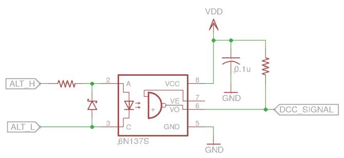
Figure 1: Opto-isolated DCC Booster Input Circuit Example
