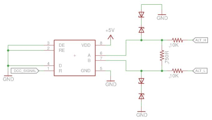
Figure 2: High Impedance DCC Signal Consumer Input Circuit Example
