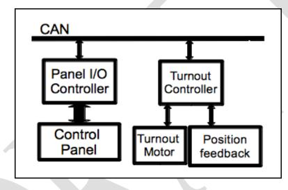
The diagram shows CAN as the transport, but a layout could also Wireless, Ethernet ,WiFi or be a combination of several technologies in the future. A layout may have, for example, a lengthy CAN
